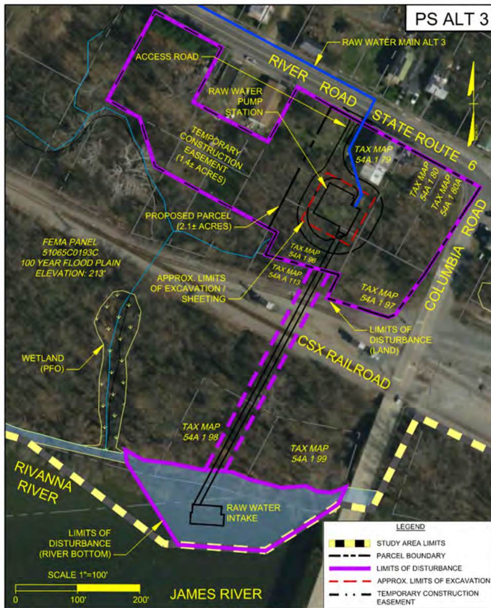
Figure 17. Build Alternative 3 Pump Station Plan View
