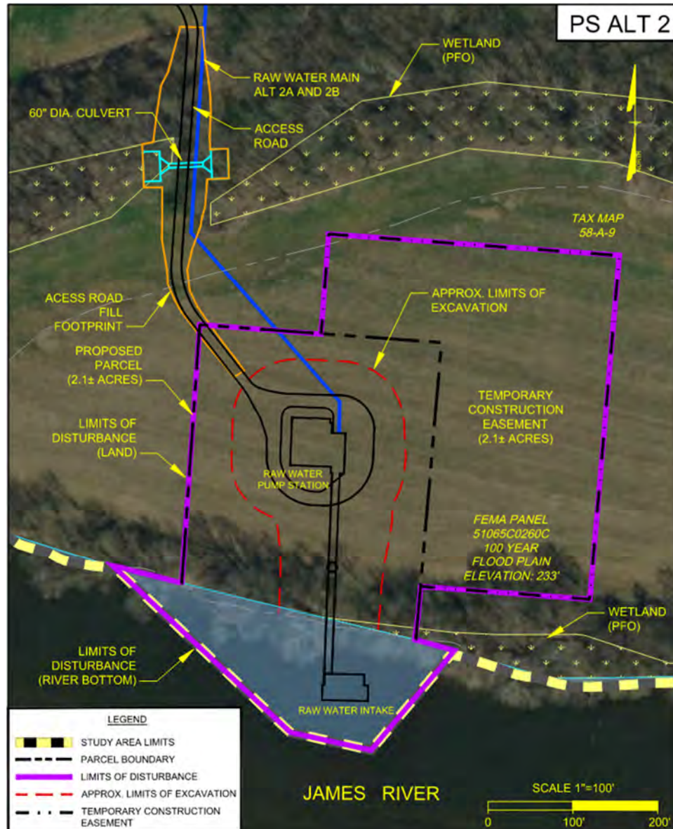
Figure 16. Build Alternative 2 Pump Station Plan View
