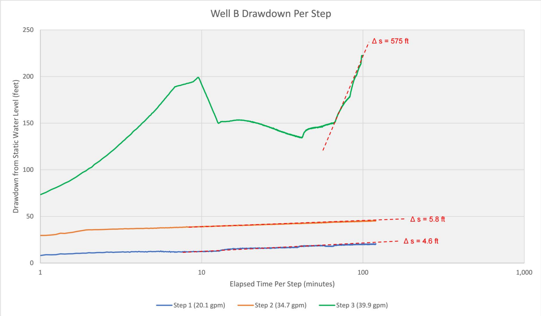
Graph B-4: Well B step-drawdown pumping test data on a per step basis.
