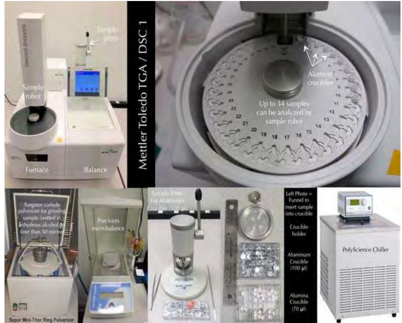
Fig. A9: Mettler-Toledo simultaneous TGA/DSC1 unit in CMC that can accommodate 32 samples. The top left photo shows the TGA/DSC1 unit with sample robot for automation as well as the sample holder for pressing aluminum sample holders. Sample is pulverized in a ring pulverizer shown in the bottom left, then a small amount (usually 30-70 mg) is weighed in a precision balance (shown 2 nd from left in bottom row) and taken in an alumina sample holder (without lid). For DSC measurements up to 600°C, sometimes sample is taken in an aluminum holder and pressed in sample press (3 rd from left in bottom row) and pierced with a needle for release of volatiles from decomposition. A PolyScience chiller (rightmost one in the bottom row) is used to cool the furnace. An ultrapure nitrogen gas is purged through the system during analyses.
